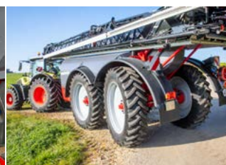
A self-steering system for one axle and an active steering for both axles are available
