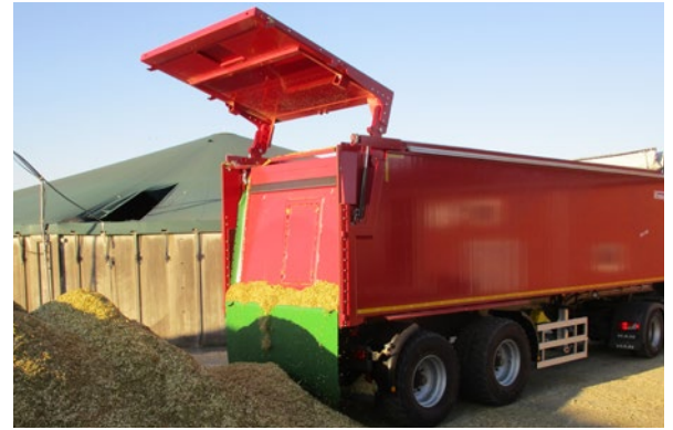
On this picture: horizontal unloading by the walking floor, optionally available with partition wall
