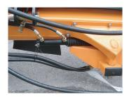
The material supply is steered hydraulically via a mobile slidegate valve.
