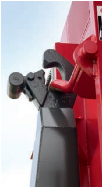
The hook mount has neatly rounded contours. A height-adjustable hook is available.
