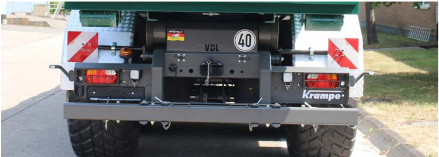
The large LED rear lights are installed in a solid protective housing.
