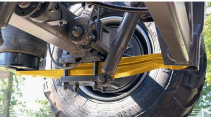
For large-volume containers with a high centre of gravity and in very bumpy terrain, we advise running gear with double-spring supports for an improved stability.
