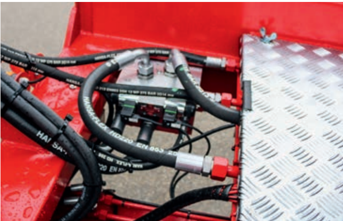
The LS block ensures faster cycle times. A rapid mode is advised as an alternative for the version with wireless remote control.
