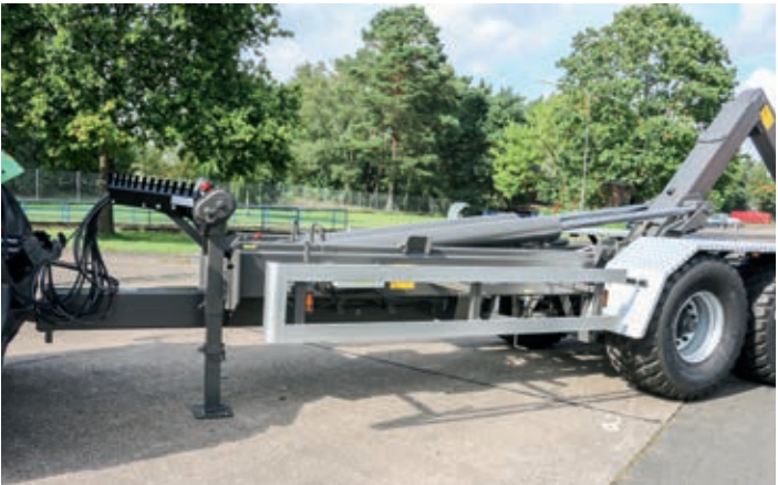
The lateral underride guard is obliged in many countries and increases safety in road traffic.
