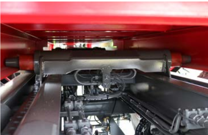
A hydraulic container locking mechanism is part of the standard equipment. Very important: This means containers of various lengths can be locked at any position.
