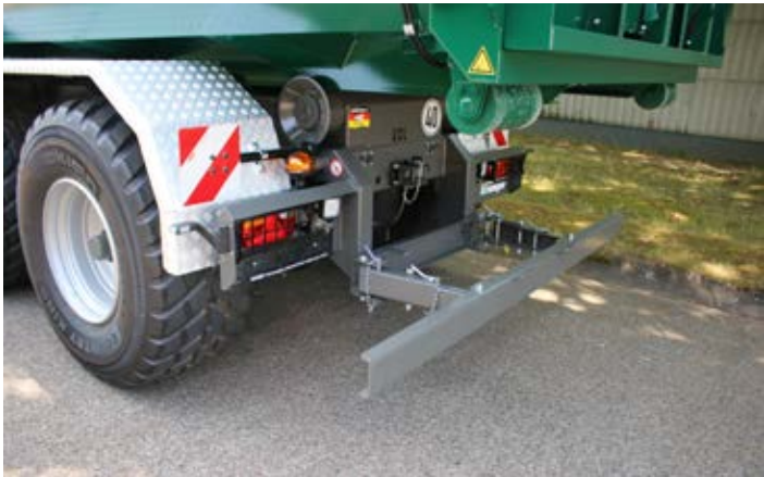
The foldable underride guard (effective stroke 50 cm) also allows the transport of extra-long containers.
