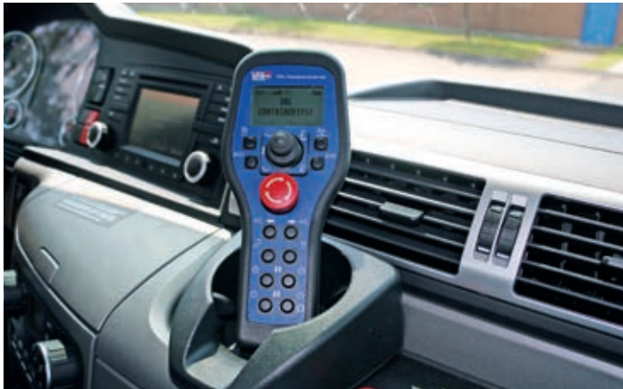
The main working cylinder, the push arm and the hydraulic container locking mechanism are very easy to operate with the proven wireless remote control. Other functions, such as rapid mode, additional control units or work lights, make the job easier.
