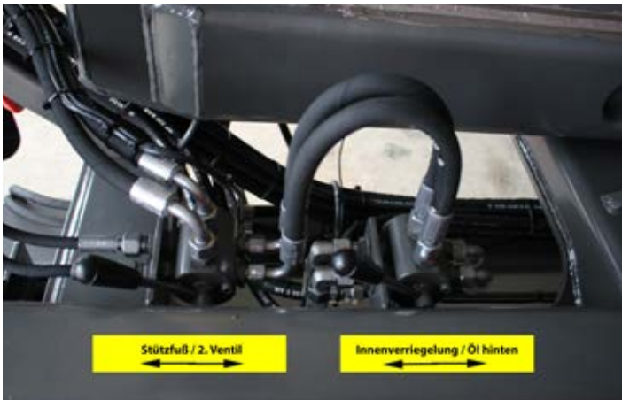
Two hydraulic functions can be operated with one control unit using the 6/2-way valve.
