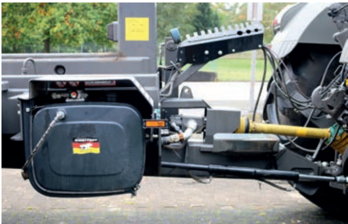
The tractor hydraulic system (200 bar) is sufficient for all roll-off tipper with a lifting power of up to 25 t. An integrated oil supply with PTO shaft is available on request. A wireless remote control is included in the scope of delivery.
