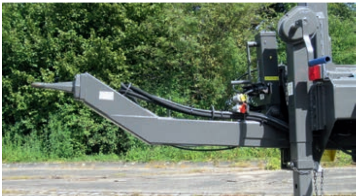
The height-adjustable drawbar (option) is suitable for all hitch heights (THL 8 L or THL 10 L).
