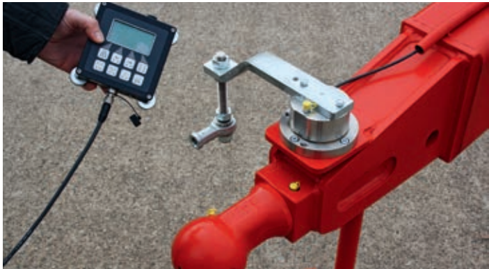
With the electrically-controlled forced steering, the driver can deliberately control the steering of the trailer thanks to different modes.
