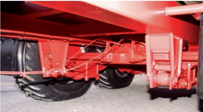
The construction height is very low in the version with parabolic suspension springs underneath the axles. A hydraulic rear axle support relieves the load on the towing vehicle during the pick-up process.
