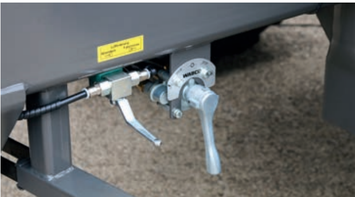
The air suspension is equipped with a reverse tap as standard. This prevents the running gear from lowering during the tipping process. As an option, a lift/lower valve can also be installed.
