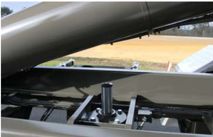
The start tipping cylinder makes it easier to tip the container when lowered. This is particularly useful when a short overhang is required during tipping.
