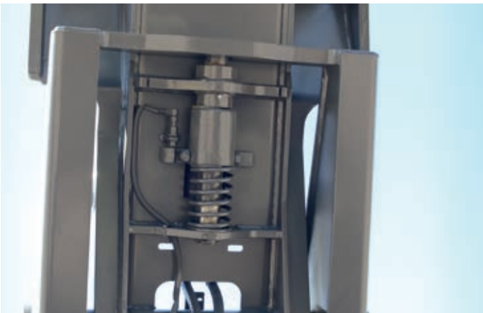
Operating errors ruled out! The container can only be set down when the push arm is fully retracted. Otherwise the lowering frame is automatically locked with the tipping frame.
