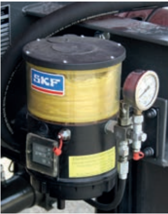
All lubrication points including those that are difficult to access are automatically supplied with grease from the central lubrication system.
