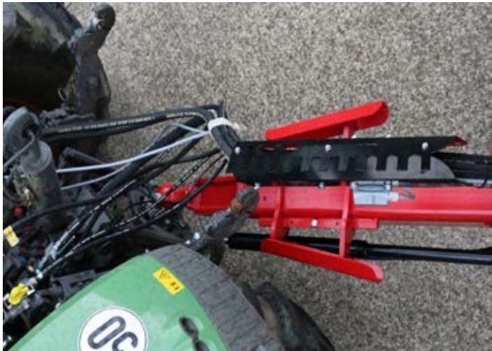
Our drawbars feature extremely slim designs that make for very tight turns. In addition, a forced steering system keeps your trailer on track at all times, at high speeds, in boggy terrain and when reversing. Moreover, it reduces tyre wear and running gear stress and strain.
