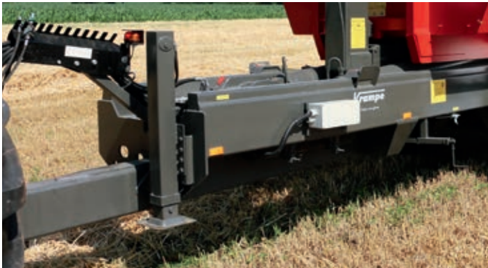
A hydraulic support foot makes hitching and unhitching the trailer easier and speeds up parking.
