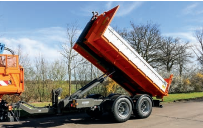
The steep tipping angle of 47–55° (depending on the model) caters for all requirements. Almost no manufacturer offers such an extensive range of roll-off tipper and special accessories. Benefit from our decades of experience.
